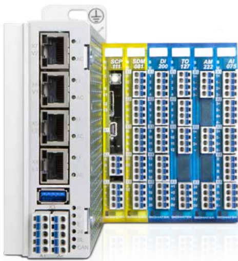
The CP 731 with a high-performance Intel® Atom™ dual-core processor.
