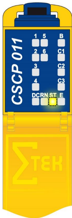
Fig. 13 Safety CPU in check configuration mode
