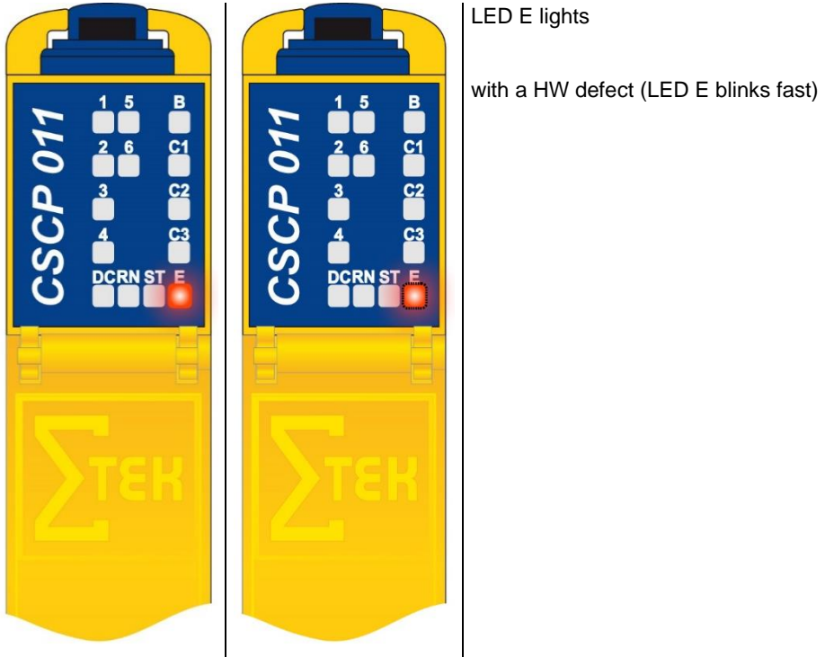
Fig. 17 Safety CPU in error mode
