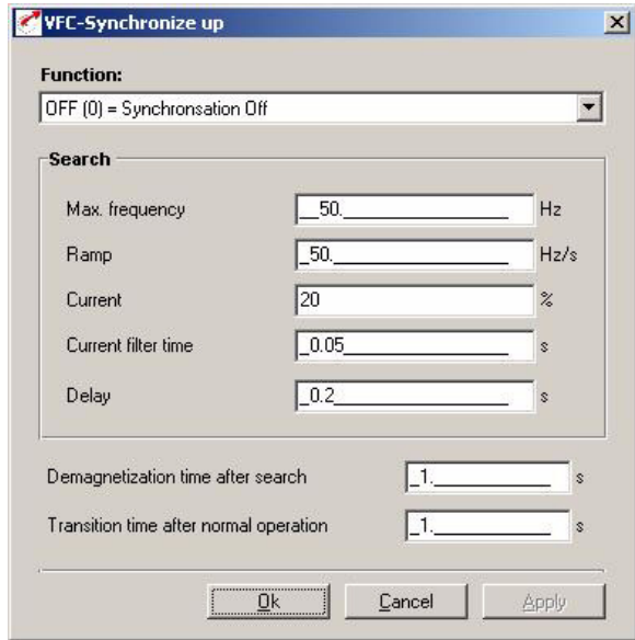
Figure 6.16 Adaptation of Up synchronization
