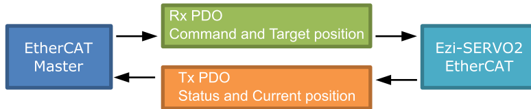
Figure 3.2: EtherCAT PDO Communication
