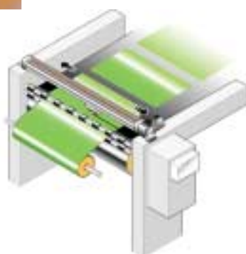
Slitting Machines High speed traverse applications for slicing of materials
