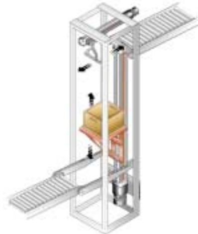
Material Handling Systems Vertical and horizontal transfer movements
